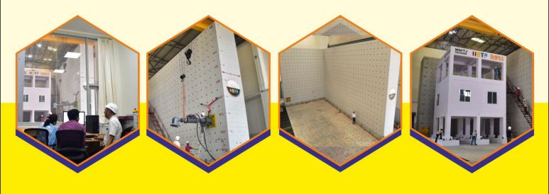
The National Earthquake Testing Facility (NETF) at MNIT Jaipur is a unique and State of the Art Testing Facility for Seismic Performance Assessment of Full-Scale Structures (quasi-static, reverse cyclic and pseudo-dynamic loading conditions) especially:
