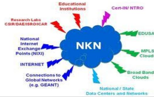
Network will consist of an ultra-high speed Core (multiples of 10Gbps and upwards), and over 1500 nodes. It is scalable to higher speed and more nodes also. The Core shall be complemented with a distribution layer at appropriate speeds. The participating institutions can directly or through distribution layer connect to the National Knowledge Network at speeds of 100 Mbps /1 Gbps.
