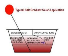
change with the natural convection of water. The bottom layer of the solar pond has a high salt content that reaches temperatures reaching 90 degrees Celsius. With the different densities in the water, the development of convection currents is prevented, which would have transferred heat to the surface of the pond, and then to the air above.
