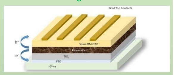
The material most commonly used for solar cells at present is silicon. However, a major disadvantage of solar cells made of silicon is the laborious and relatively costly production process involved. The most promising alternative is solar cells based on perovskites, a photovoltaic crystalline material which resembles calcium titanium oxide in terms of structure.
