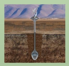
the temperature differences. It is planted six feet below the ground surface, and soil is then packed around its metal neck. The top of the Water Seer holds a vertical wind turbine, which spins internal fan blades to draw air into the subterranean chamber. Because the underground chamber of the Water Seer is cooled by the surrounding
