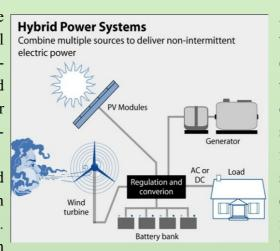
distribution system. For the times when neither the wind nor the solar system are producing, most hybrid systems provide power through batteries and/or an engine generator powered by conventional fuels, such as diesel. If the batteries run low, the engine generator can provide power and recharge the batteries.
