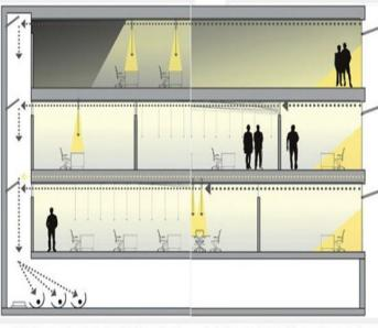
This diagram shows how SmartLight can direct ... to the inner part of a building and to a centralized sunlight from the outside of a building (far right)... to the inner part of a building and to a centralized harvesting- and energy-storage hub (far left).
