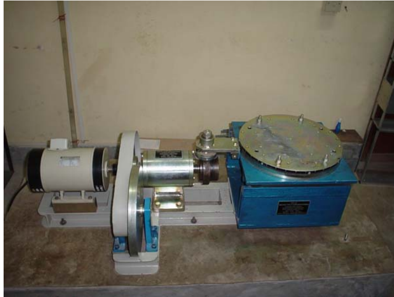
Fig 1 Electric motor driven shake table
