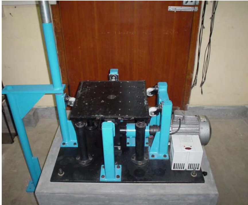
Fig 5 Electric motor driven shake table (harmonic vertical base motion).
