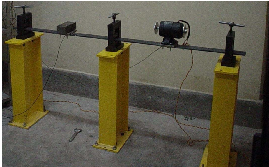
Fig 33 A view of two span simply supported beam setup.
