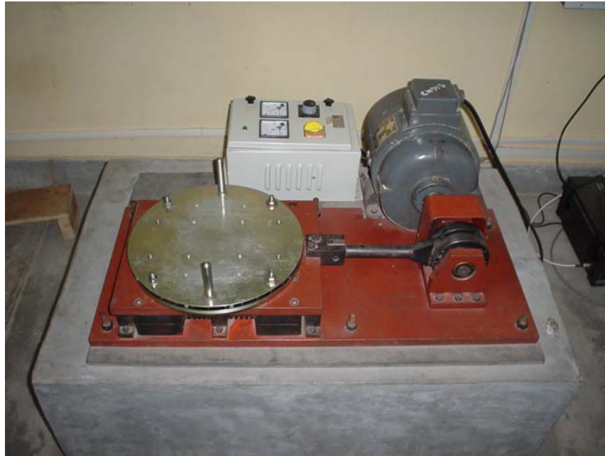
Fig 4 Electric motor driven shake table
